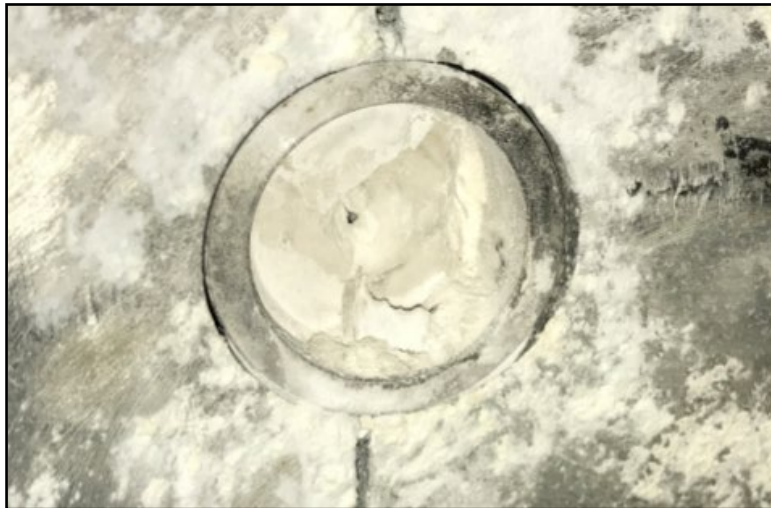
Figure 2. - Product buildup in shaft support boss
