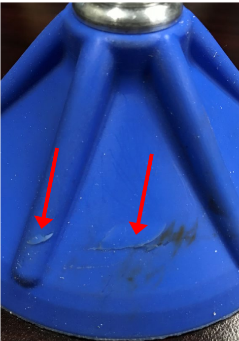
Figure 1. – Cuts into the cone.
