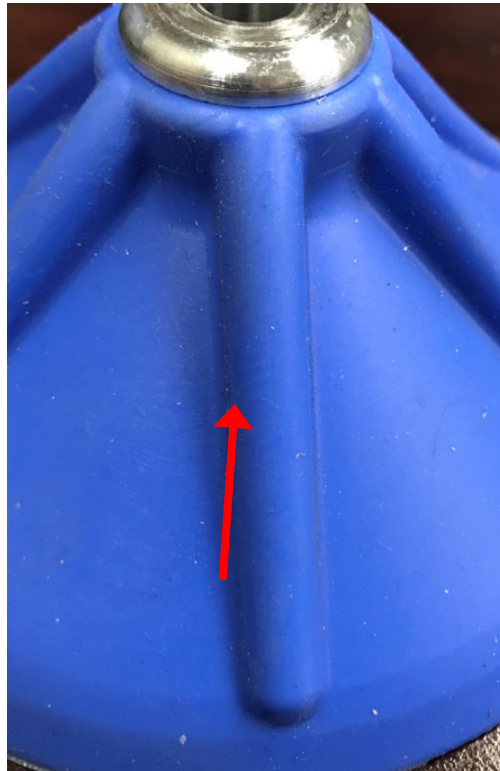
Figure 4. – A perfect cone with no cuts or tears. The cone top is also perfectly seated under the aluminum.
