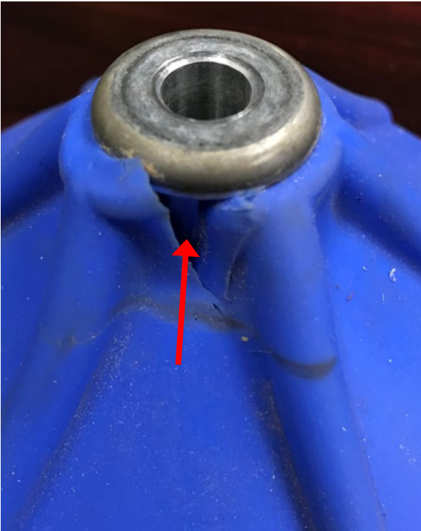
Figure 3. – Rips and tears in cone.
