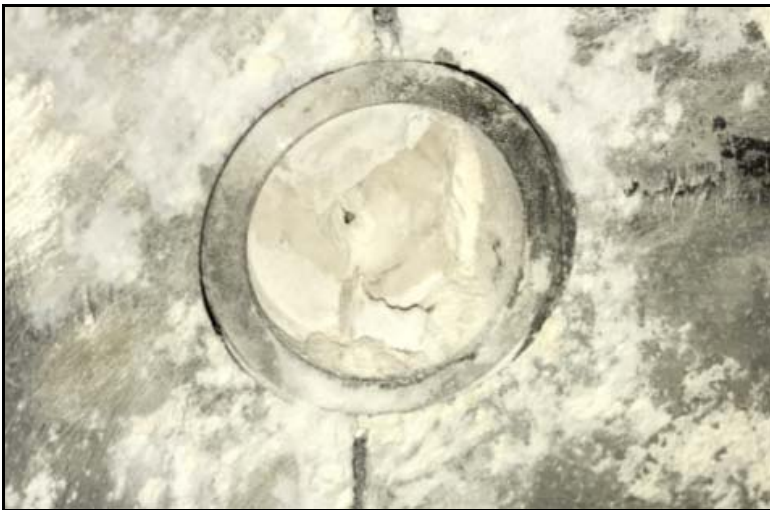
Figure 2. - Product buildup in shaft support boss
