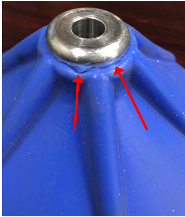
Figure 2. – Cone top not properly seated under aluminum insert bushing.
