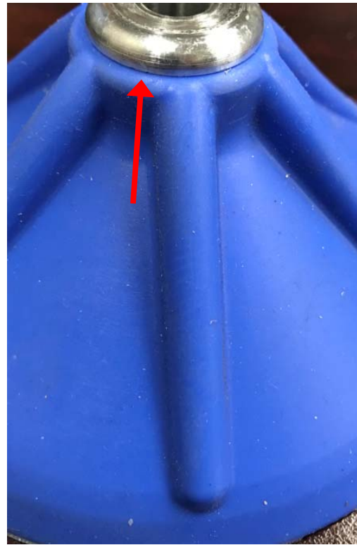
Figure 4. – A perfect cone with no cuts or tears. The cone top is also perfectly seated under the aluminum.
