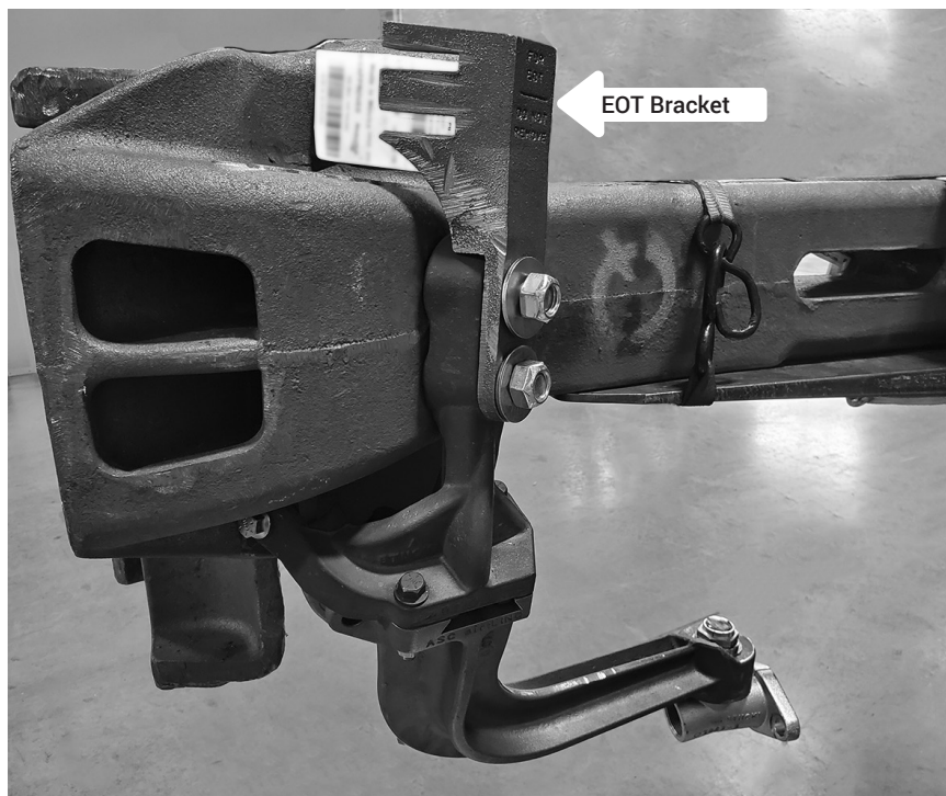
Figure 17. EOT bracket addition.
