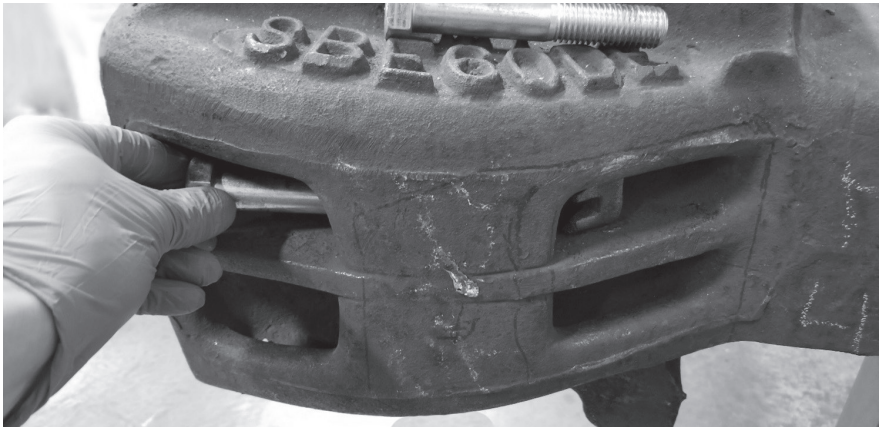
Figure 7. Image of top insert application through side of lightener hole.
