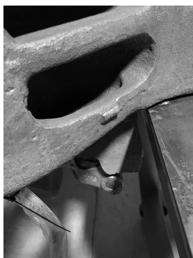
Figures 12-14. Light grinding can be done for a better fit.
