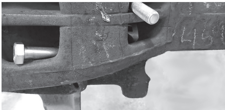
Figure 10. Image of bottom insert application through side of lightener hole.
