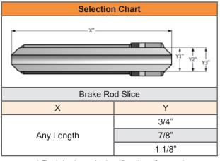
\* Each brake rod takes 2 splices for repair.
